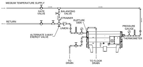
HOT WATER PIPING, 270 F AND BELOW VARIABLE FLOW THRU GENERATOR
